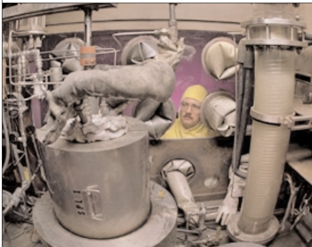
Fluor Federal Services is the prime contractor for the remediation of the Department of Energy's Hanford site in Washington. Pictured is a prototype calciner at Hanford's Plutonium Finishing Plant, which began converting corrosive plutonium solutions to a stable, dry powder for safe storage in September of 1999.
